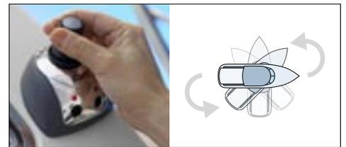
Twist the top to rotate. Combine it with any other move to compensate for wind or current.
